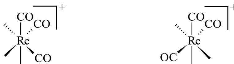
Figure 1. Complex compounds containing a [\text{Re}(\text{CO})_3]^+ core, with facial geometry (left) and meridional geometry (right). In order to increase the clarity of the figure, the remaining ligands have been omitted
